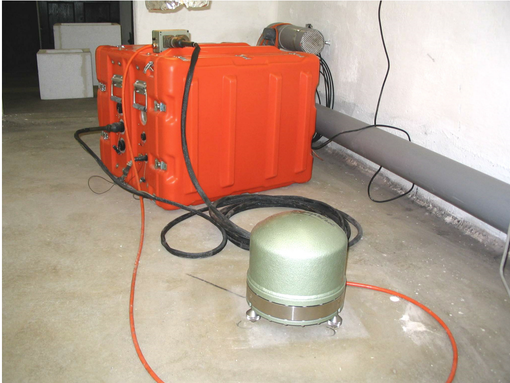
Figure 5.18: STS-2 seismometer and Quantera data logger.
