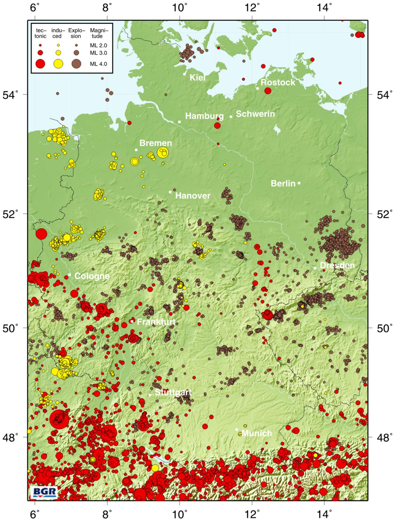
**Figure 5.3:** Seismic events with magnitude 2.0 and above in Germany and adjacent regions in the recent 20 years (1998-2017). The tectonic events, induced events, and explosions are colour coded. The different magnitudes of the events correspond to the size of the circles.
