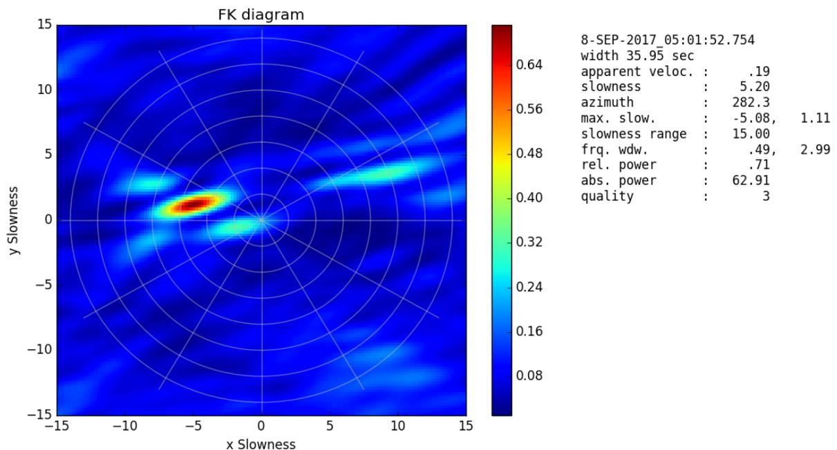
**Figure 5.4:** Result of the *f-k* analysis for the *P* wavetrain of an event offshore Mexico (08.09.2017, 04:49:21 UTC, *M<sub>s</sub>* 8.3) recorded at the Gräfenberg array. The inferred slowness and azimuth can be used to backtrack the ray and determine the epicenter.
