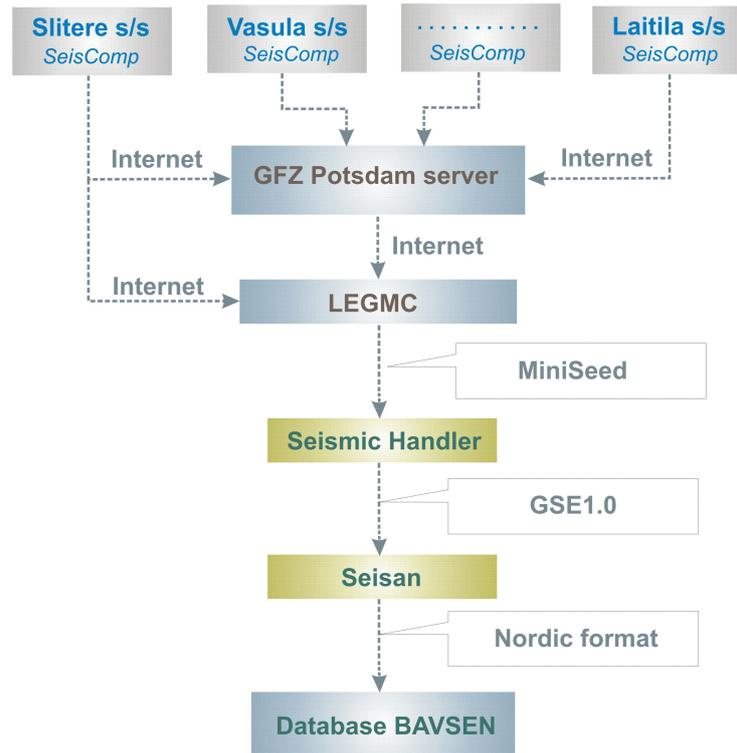
**Figure 6.11:** Flow chart of transmission of seismological information from the stations to the servers, data formats, software and processing steps.
