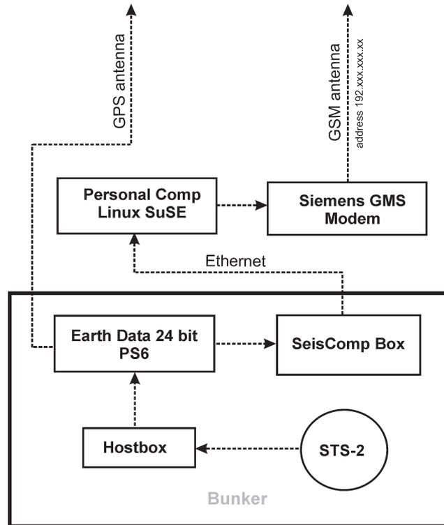
**Figure 6.10:** Scheme of typical equipment of a GEOFON seismic network station.
