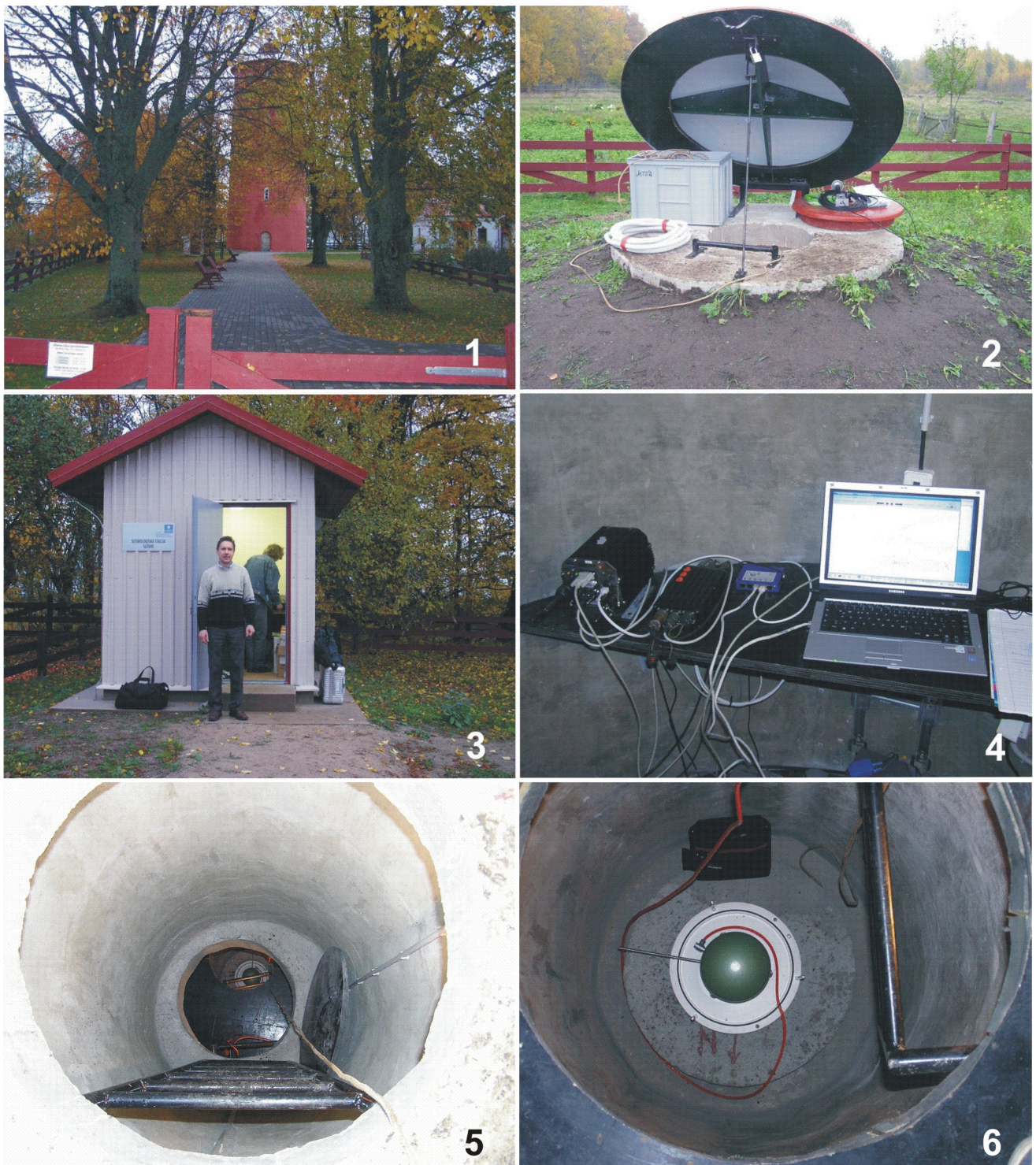
Figure 6.9: Seismic station Slitere (Latvia). 1 - lighthouse "Slitere"; 2 - entrance to the instrumental bunker; 3 - tool house; 4 - SeisComp unit and analogue-to-digital converter PS6 Earth Data 24; 5 - a view of the STS-2 sensor from the height of the upper compartment; 6 - a view of the STS-2 sensor from the height of the middle compartment.
