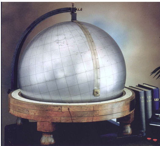
Figure 2.1: The steel globe bearing positions of early seismic stations was used for locating positions of earthquakes for the International Seismological Summaries .
