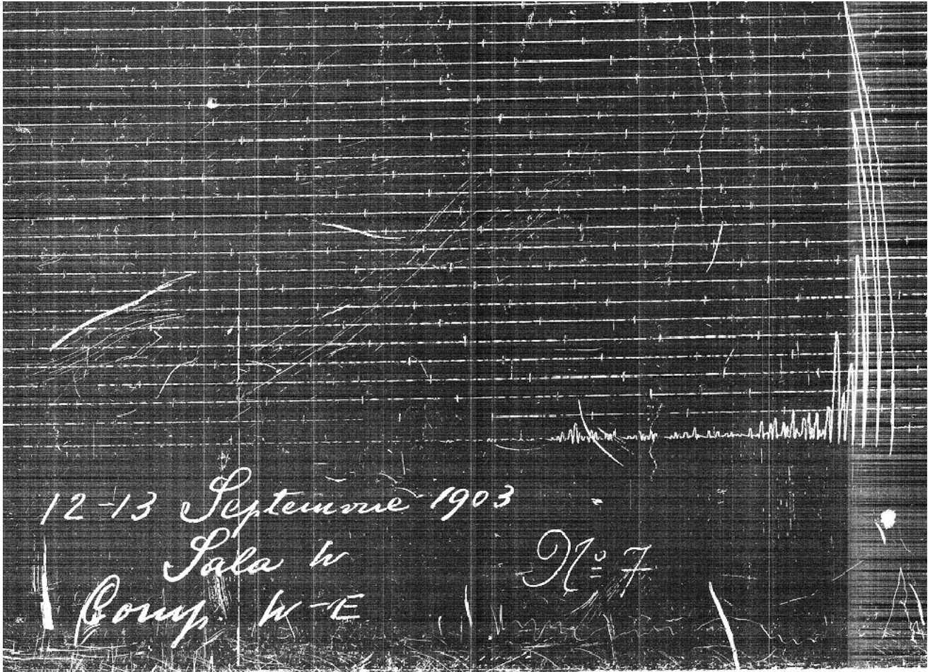
Figure 6.3: Bosch mechanical pendulum seismogram recorded by the EW component for the Vrancea earthquake of 13 September 1903 at 10:02 GMT ( M = 6.3 ). Half of the motion trace is available (scanned seismogram).
