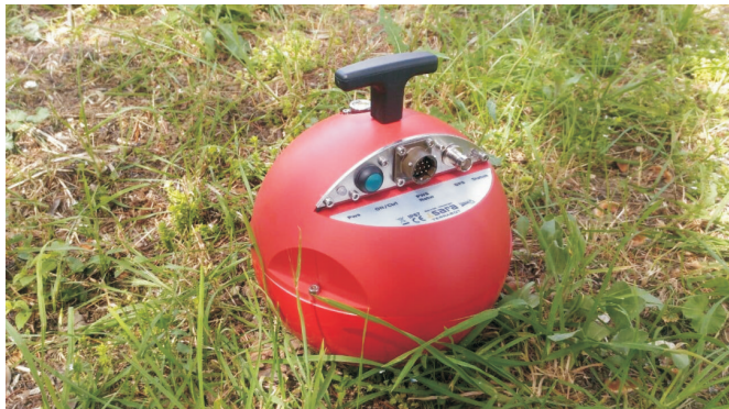
Weak motion sensor and microtremor (HVSR) Nodal systems - Terrabot
