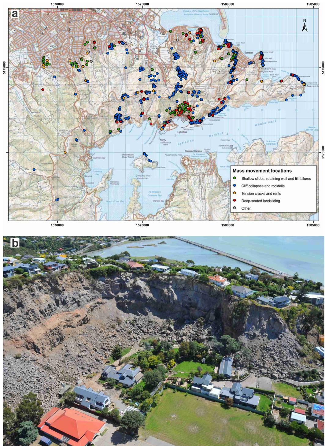
**Figure 8.8:** (a) Map showing the distribution of mass movements caused by the Christchurch earthquake (from Massey et al. 2014). (b) Example of earthquake induced mass movement showing the proximity of homes at the top and base of the cliff, photographer Graham Hancox, copyright GNS Science/EQC, VML ID 130503.
