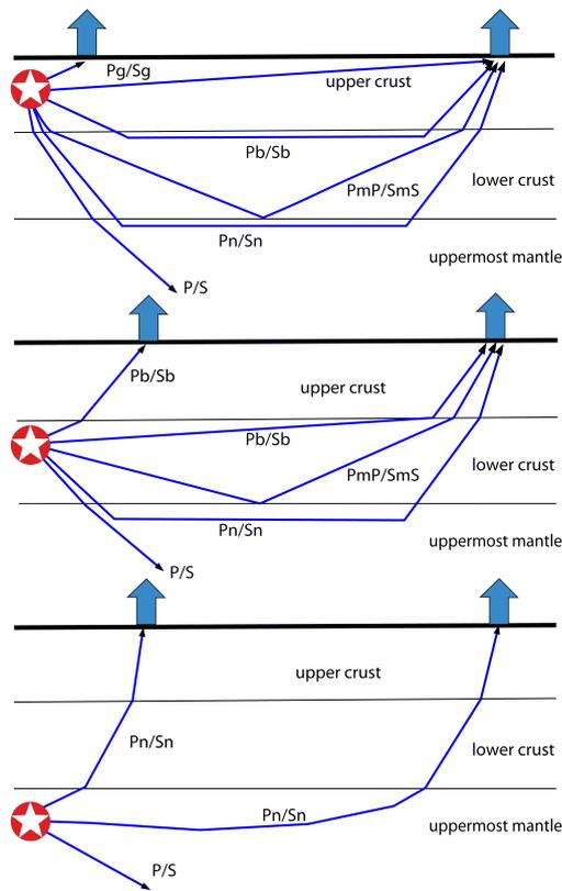
**Figure 6.1:** Seismic ‘crustal phases’ observed in the case of a two-layer crust in local and regional distance ranges ( $0^\circ < D < \text{about } 20^\circ$ ) from the seismic source in the: upper crust (top); lower crust (middle); and uppermost mantle (bottom).
